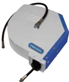
29 473 Hose reel, water/air, encased, GDA, for wall/floor mounting, 20 bar, DN 10, 15 m
