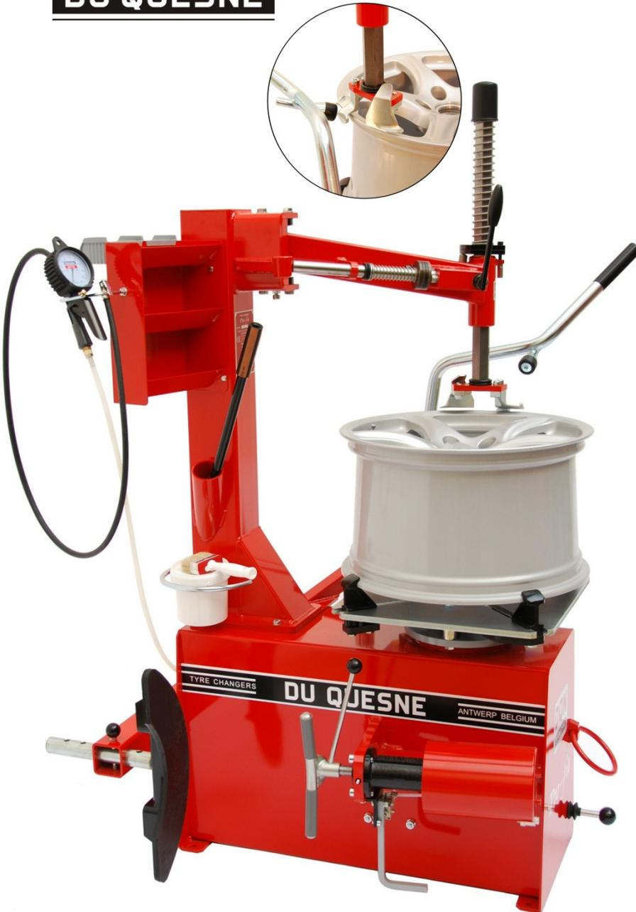
1. The **LINEAR BEAD-BREAKER** with telescopic pre-adjustment of the pressure plate is designed to prevent any damage either to the rim or to the tyre. Its power even makes it unnecessary to deflate small tubeless tyres before bead breaking.
